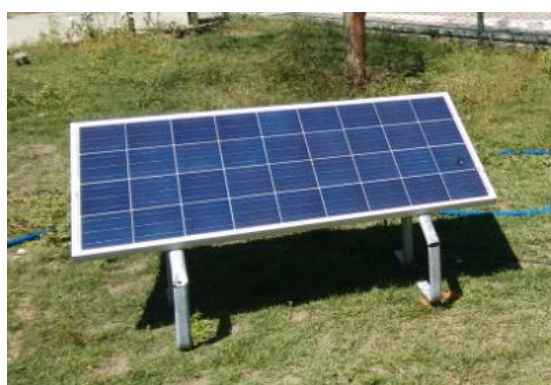
Figura 2: Paine solar Yingli YL140P.
